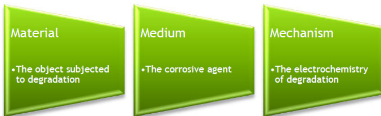
Fig. (1). The 3 Ms of corrosion.
