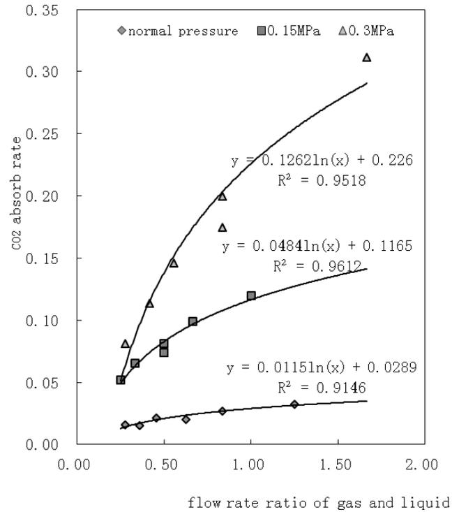
Fig. (3).  $CO_2$  solubility changing under different scrubbing pressure condition.
